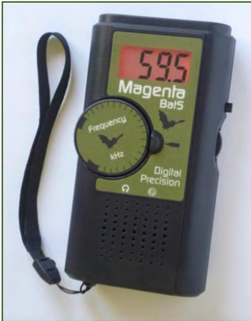
The Magenta Bat5 is a superheterodyne bat detector with an illuminated, easy to read (day or night), 4-digit LCD frequency display. It has a range of 10kHz to 130 kHz and an extended low frequency range suitable for insects and some birds.
